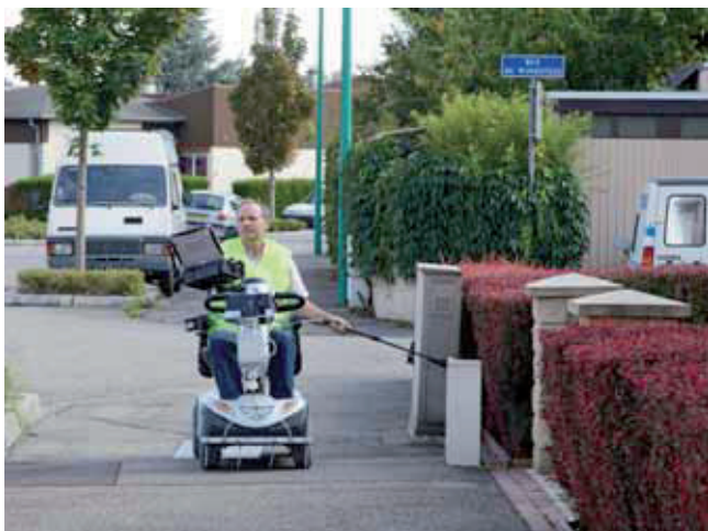
Figure 3. The ECO INSPECTRA® vehicle was developed by GAZOMAT™ for survey of pedestrian areas not accessible to a traditional network survey vehicle.
