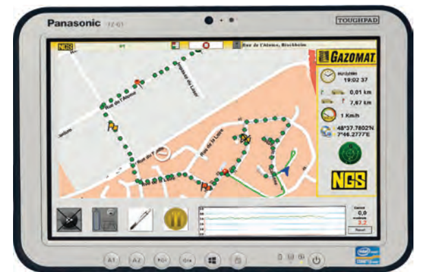
The NGS survey software installed on a PC or PC tablet provides real-time visualisation of the survey circuit with continuous display and recording of gas leak detected and survey events along with associated GPS co-ordinates.
