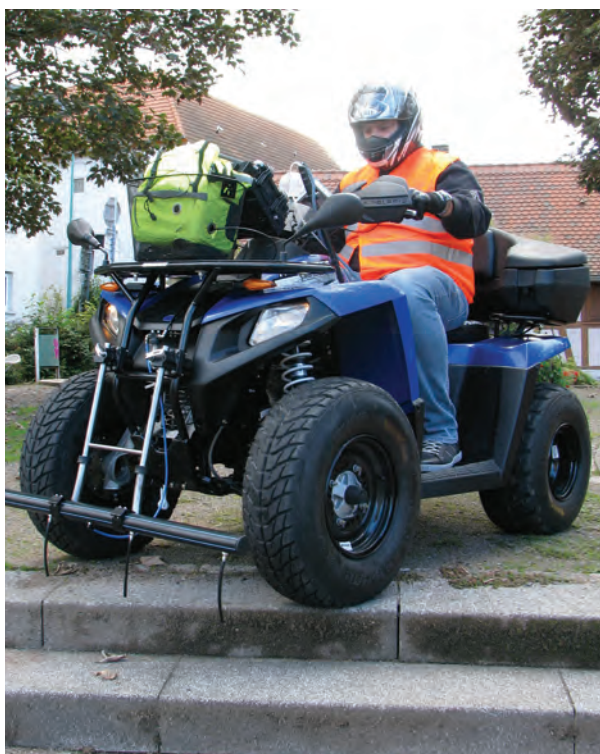
The EASY INSPECTRA™ mounted on an ATV makes it possible to survey gas transmission pipelines or off-road areas.
