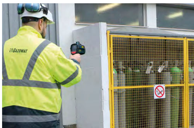
Figure 2. The GAZOSCAN is a handheld remote methane leak detector. It connects wirelessly to a mobile phone and transfers readings to the GAZOSURVEY application.
